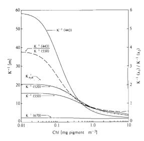
Fig. 3. Penetration depth,  $Z_{900} \approx K^{-1}$  (m), versus chlorophyll concentration, C (mg. m<sup>-3</sup>) as derived from an optical classification model (Smith and Baker, 1978b; Baker and Smith, 1981). Penetration depth calculated for 4 CZCS spectral bands  $K_{igl}^{-1}$  and for total photosynthetically available radiant energy,  $K_{FAR}^{-1}$ . Scale on right ordinate gives ratio of penetration depth in blue band to that in the green,  $K_{-1,300}^{-1}$
