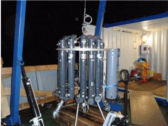
Fig. 2. CTD with rosette 12 Niskin bottles and one 20 L Go-Flo mounted. All non-stainless steel parts of the system were covered in plastic (Photo Per Andersson).
